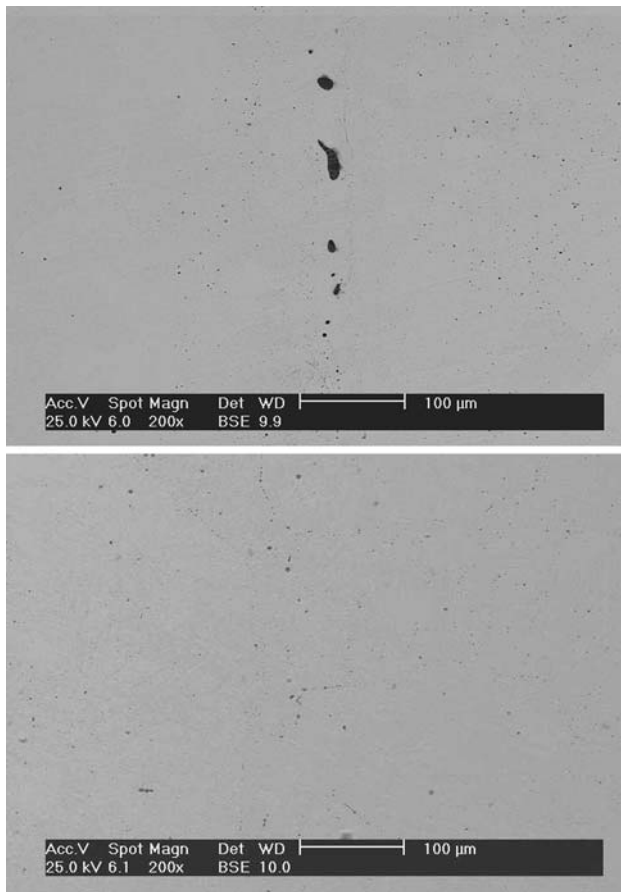
Fig. 2 Scanning electron micrographs (back scattering electron detection) of the union zone for steel/iron-boron/steel bonding at 1,250 °C. The joints were performed under applied pressures of 2 MPa (top) and 4 MPa (bottom). The process time is 7 min
